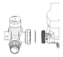
1.2 Install the gasket into the connecting nut of the water supply system component, and then match the connecting nut with the external thread of the water pump and tighten it. Ensure that water supply system components, gaskets and pumps are in sealed fit.
