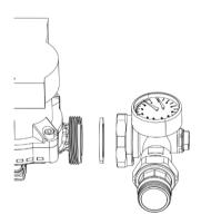
1.3 Swivel out the male unions of the mixing system and supply system, rotate its 1" male threads into the main bar or 1" female threads of other control unit, use the cone ring or other sealing winding belt of the tubes to tighten and seal, then re-rotate the free nut of the union into the mixing system and supply system correctly to avoiding leaking.
